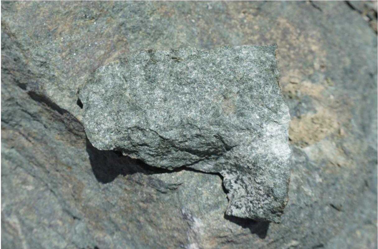
Outcrop IV, Greenstone, meta-basalt or metagabbro probably containing chlorite
